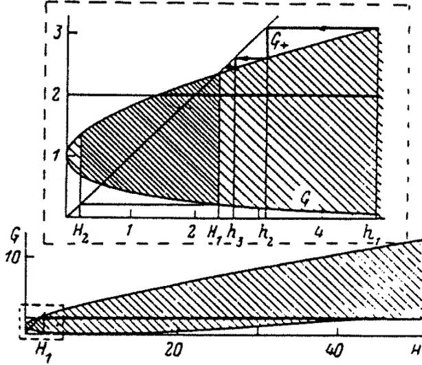
Figure 2: Integration interval in Eq. (17) is a segment of the the horizontal line located in shaded region (in the search for transition distributions) or in the dark-shaded region (in the search for a stationary distribution). Top shows enlarged image of rectangle bounded by shading lines.
